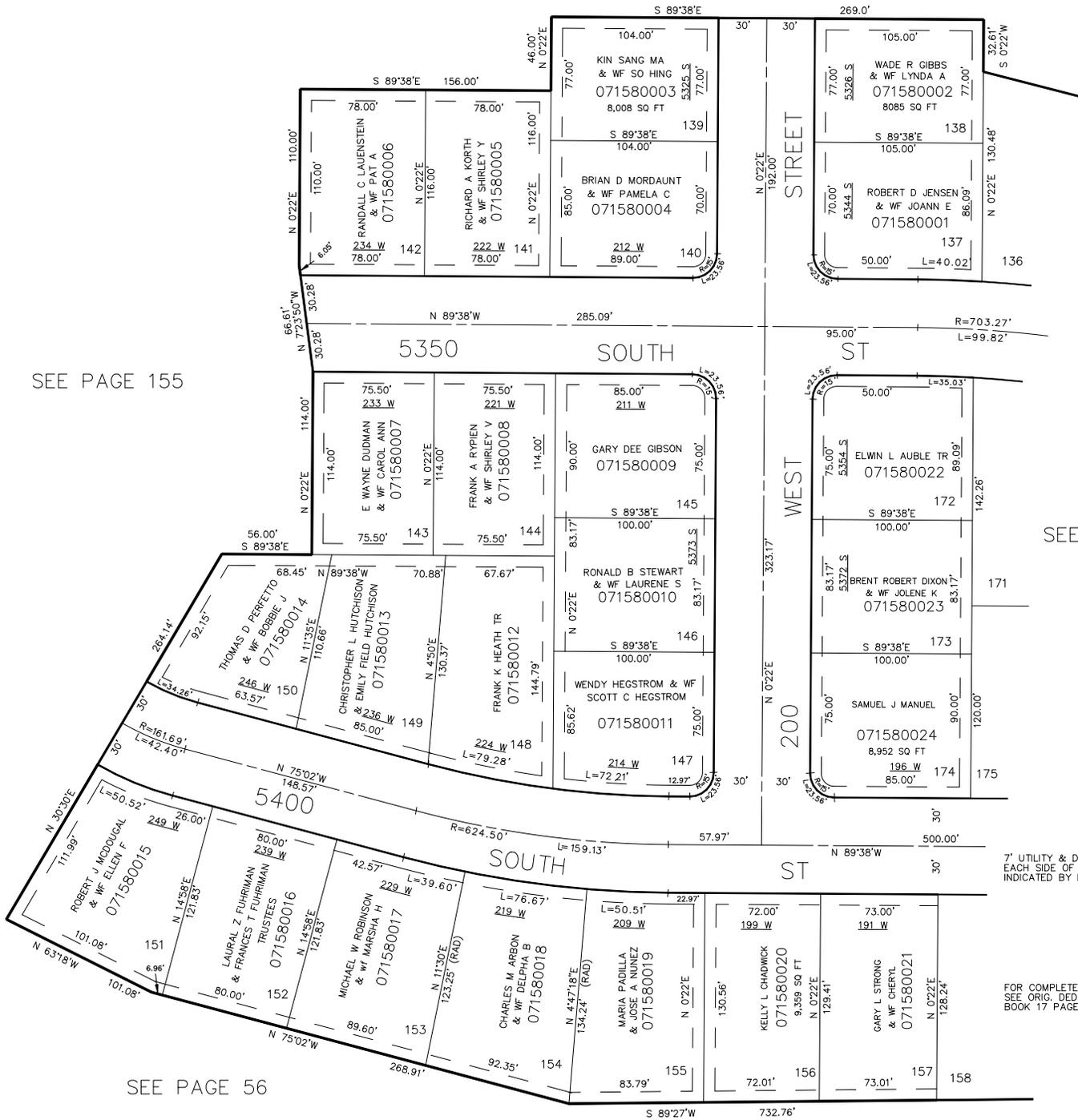
7' UTILITY & DRAINAGE EASEMENTS EACH SIDE OF PROPERTY LINES AS INDICATED BY DASHED LINES.
